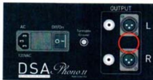
Figure 8 – Location of switch and holes for polarization balance
